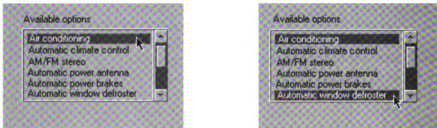
Figure 67. Random-point Selection. During random-point selection a user selects several items in any order. The items do not have to be contiguous.
